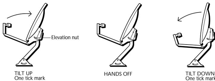
8. When you achieved what you believe to be the highest signal strength (peak signal), tighten the elevation nuts on the support arm.
