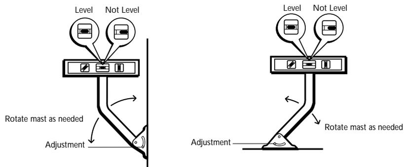
**Step 2:** Verify that the mast is level front-to-back.
