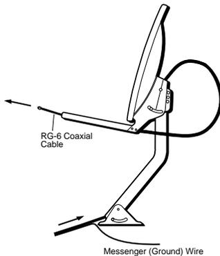
**Step 3:** Route the cable through the mast.
