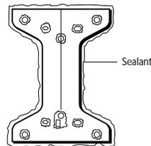
**Step 11:** Seal the mounting foot to avoid water leakage.
