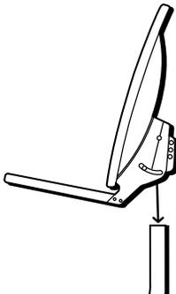
**Step 1:** Place the dish assembly on the mast or pole
