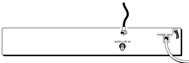
**Step 2 & 3:** Take the phone off the hook before you connect a phone cord from an outlet to the back of the receiver.
