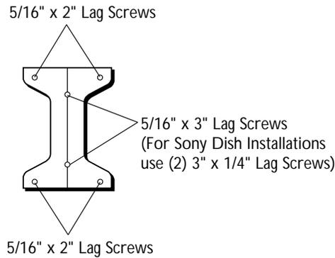
**Steps 8 & 9:** Inserting the lag screws.
