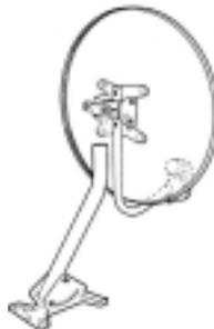
**Sony Step 1:** Loosen the mast clamp and lower reflector onto the mast. Tighten the clamp screws.
