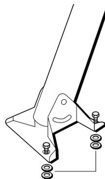
**Step 3:** If the mast is not level, add washers to level the foot.
