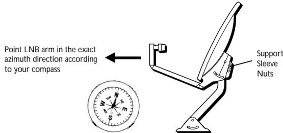
2. If you do not hear a continuous tone from the signal meter, use the following procedure to adjust the dish until you hear one continuous tone:
