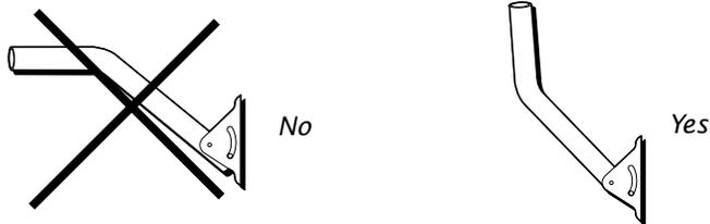
**Step 7:** Make sure that the top of the mast will point straight up.
