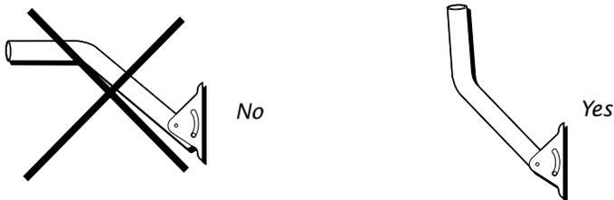
**Step 8:** Make sure that the top of the mast will point straight up.
