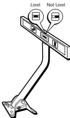
**Step 2:** Verify that the mast is level side-to-side.
