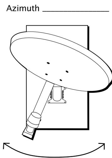
*Azimuth is side to side direction that the dish is pointed*
