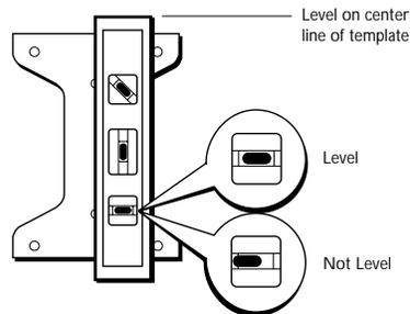
**Steps 2 & 3:** Center the mounting on a rafter and make sure that it is level.
